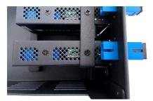
When all the EXT-DP12-OPT optical extenders have been installed, tighten the 5 screws of the extenders mounting bracket on the front panel.
